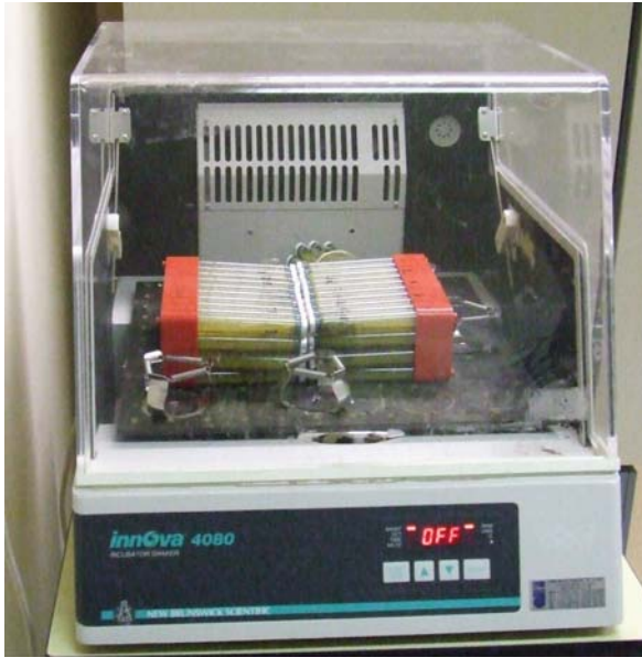
Fig. 9.11 Orbital shaking incubator with Belco tubes placed horizontally
