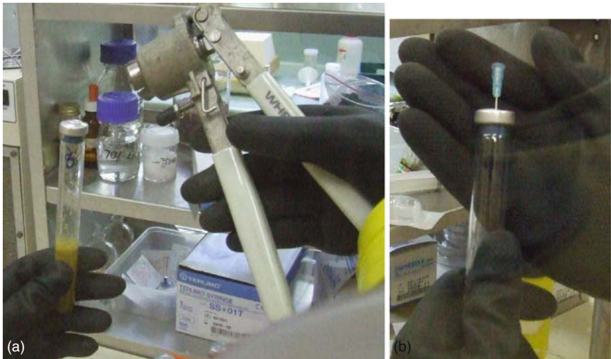
Fig. 9.10 (a and b) Sealing and venting Belco tubes
