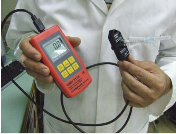
Fig. 9.5 Pressure transducer (Greisinger GMH 3110)
