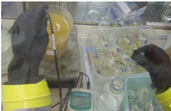
Fig. 9.19 Bringing the pH to 7 using 3N HCl in the anaerobic chamber
