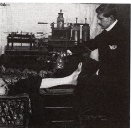
Early X-ray photography of a leg in 1896. The picture that was produced was called a skiagram.
