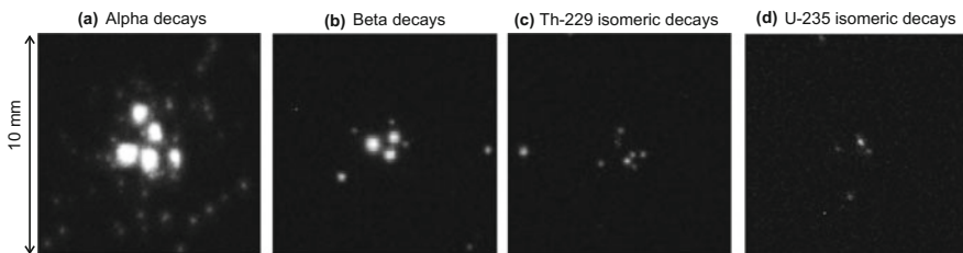
Fig. 5.21 Different classes of decay events as observed during ion accumulation on the MCP surface (Beam Imaging Solutions, BOS-75-FO) [6]. Individual frames of 4 s exposure time at an MCP surface voltage of -25\ \text{V} are shown. The extracted ion species was chosen by mass-to-charge separation with the QMS. a \alpha decays originating from ^{221}\text{Fr} ( t_{1/2} = 4.8\ \text{min} ). b \beta decays originating from ^{209}\text{Pb} ( t_{1/2} = 3.25\ \text{h} ). c ^{229}\text{Th} isomeric decay ( t_{1/2} \approx 7\ \mu\text{s} ). d ^{235}\text{U} isomeric decay ( t_{1/2} = 26\ \text{min} ). With kind permission of Nature Research [6]
