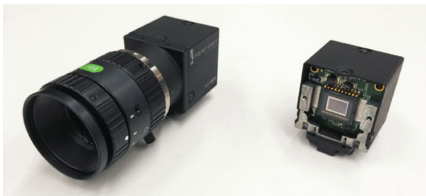
Fig. 4.30 Photograph of the CCD camera (Point Grey, FL2-14S3M-C) combined with a zoom lens (Computar M2514MP2, 25 mm, C-mount) used for read-out of the MCP detection system (left). The right-hand side shows the CCD chip (Sony, ICX267 CCD) of an open camera. (Photograph from Ref. [48])
