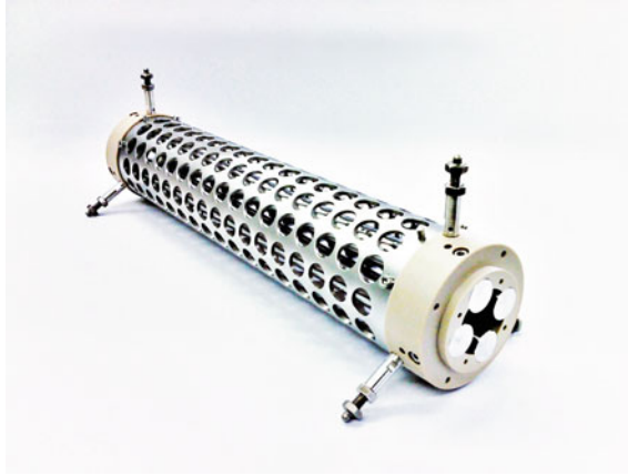
Fig. 4.13 Photograph of the quadrupole mass-spectrometer (QMS) required for ion-beam purification. The QMS was developed following design values given in Ref. [17]. The production of a mass-purified ^{229}\text{Th} ion beam is a prerequisite for the unambiguous identification of the isomeric decay. Otherwise, short-lived decay products of the ^{233}\text{U} and ^{232}\text{U} decay chains could not be excluded as signal origin. With kind permission of The European Physical Journal (EPJ) [16]
