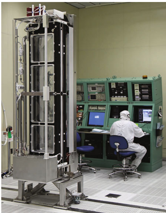
Fig. 10.42 Plasma-electrode Pockels cell module for NIF. Lawrence Livermore National Laboratory
