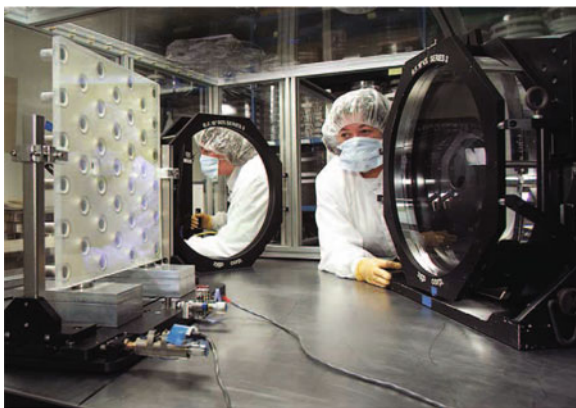
Fig. 10.41 Deformable mirror used on the NIF. Lawrence Livermore National laboratory
