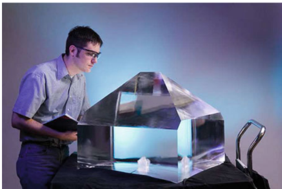
Fig. 10.40 Large format KDP crystal for NIF. Lawrence Livermore National Laboratory
