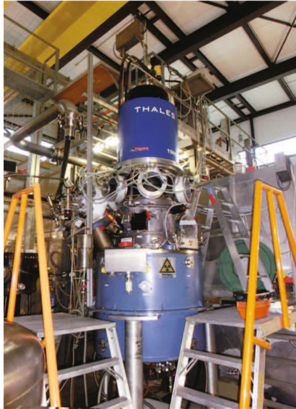
Fig. 9.60 Prototype 170 GHz gyrotron for ITER from Thales Electron Devices. ©2015 European Joint Undertaking for ITER and the Development of Fusion Energy (“Fusion for Energy”)
