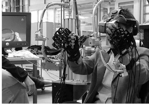
Fig. 8.8 VR testing lab with haptic feedback (Reprinted from Kuhlen and Jerabkova [65])
