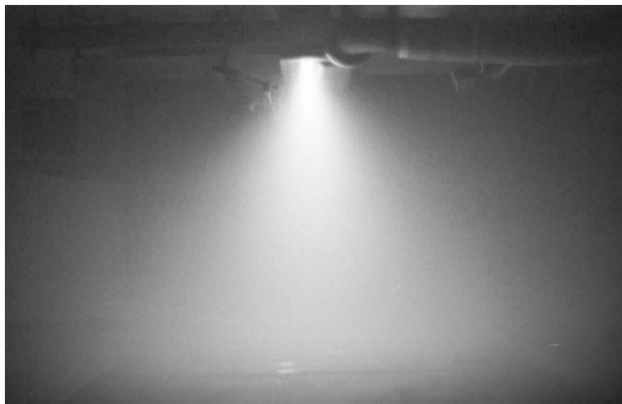
Fig. 1 Visible light glow indicates that the cold plasma is formed inside the process vessel in which gas is irradiated (pilot plant at EPS Kaweczyn, Poland)
