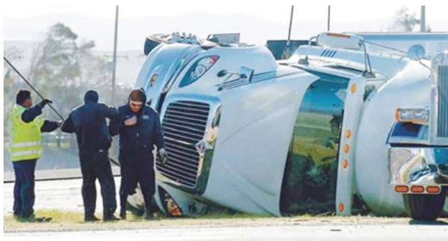
Fig. 18.3 Tow truck workers hook a tractor-trailer close to San Bernardino, CA, overturned by strong cross-wind gust on February 2nd, 2011 (Photo courtesy of Jennifer Cappuccio Maher)
