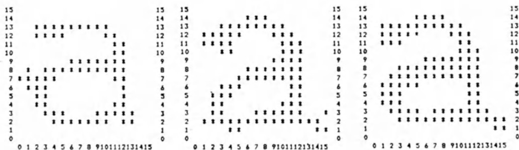
FIG.9:Some examples of masks as obtained by cluster analysis. A pseudo-distance is evaluated for each pair of samples. A group of samples is taken as valid if no pseudo-distance exceeds a prefixed threshold. A dot of a mask is black when it is black in more than a certain amount of samples belonging to the corresponding group.
