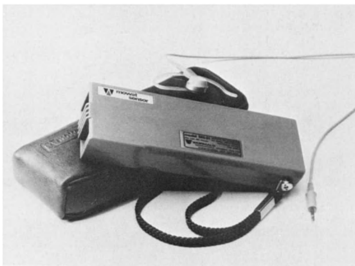
Fig. 1. Mowat Sonar Sensor. (Wormald International Sensory Aids)
