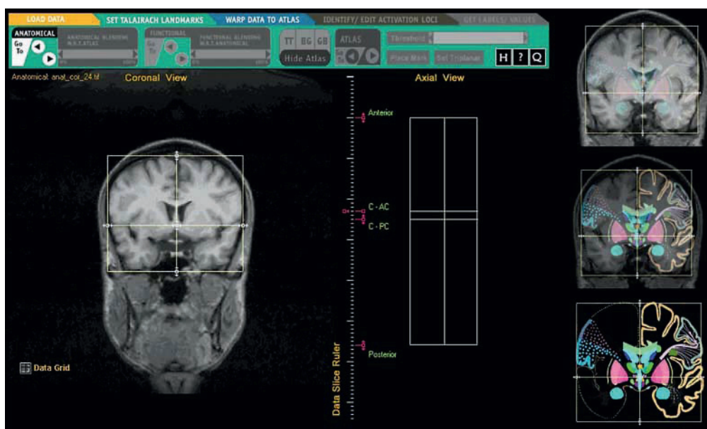
Fig. 8.17. Screenshot from the Brain Atlas for Functional Imaging (BAFI) (NOWINSKI and THIRUNAVUUKARASUU 2000). Showing the application of a Talairach coordinate system to a coronal image from a 3D brain MRI. After application of the coordinate space the images can be coregistered to the standard Talairach map. The images on the right show the coregistered images with varying degrees of opacity to demonstrate the image ( top ), the pure atlas ( bottom ) and a fused version ( middle )
