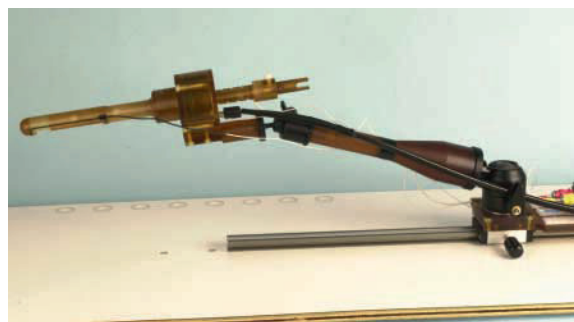
Fig. 28.10. The MR-compatible robot device, developed for transrectal prostate interventions, as assembled on the MRI table
