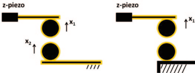
Fig. 5.8 The current experiment reduces the hydrodynamic coupling between cantilevers by keeping them well separated and antiparallel (left). A conventional drainage experiment could achieve a similar effect by attaching the bottom sphere to a step edge (right)
