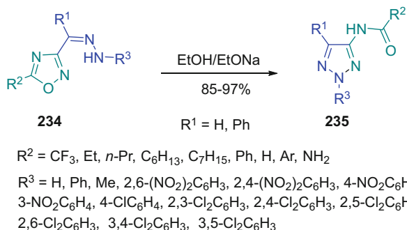
Scheme 82 Intramolecular rearrangement of the Z-aryldiazones of 1,2,4-oxadiazole 234 to 5-acylamino-2-aryl-1,2,3-triazoles 235
