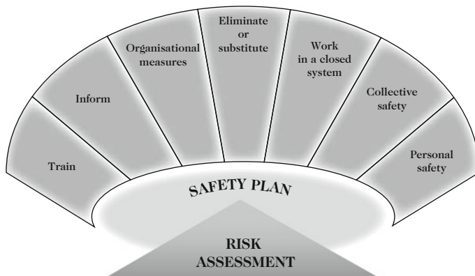
Fig. 10.1. Plan of action for implementing safety measures. Adapted from V. Causse/INRS
