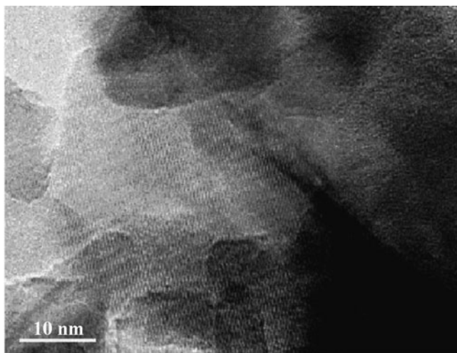
Fig. 9.2 TEM micrograph of the mechanically activated mixture for the synthesis of porous mullite ceramics after 3 h attriting (bar 10 nm)
