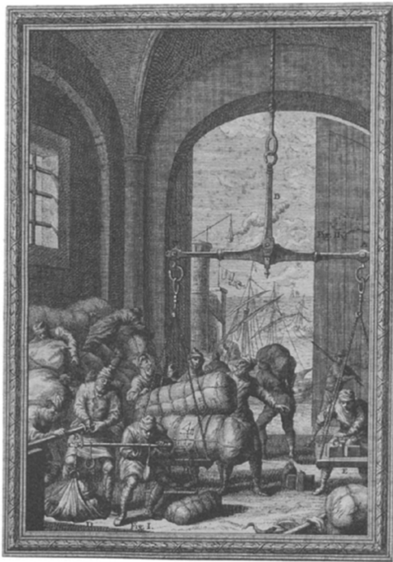
Figure 4.1 The balance and the steelyard. The illustration pictures the two means of weighing commercial goods common in the eighteenth century: the unequal arm balance or steelyard in the foreground to the left (“Fig. I”) and the equal arm balance or scale in the background at the right (“Fig. II”), the former utilizing the mechanical advantage of the lever. For a detailed discussion of these considerations see Bruno Kisch, Scales and Weights: A Historical Outline , Yale Studies in the History of Science and Medicine, no. 1 (New Haven, Conn., 1965). Note the merchant’s marks on the bales of goods.
