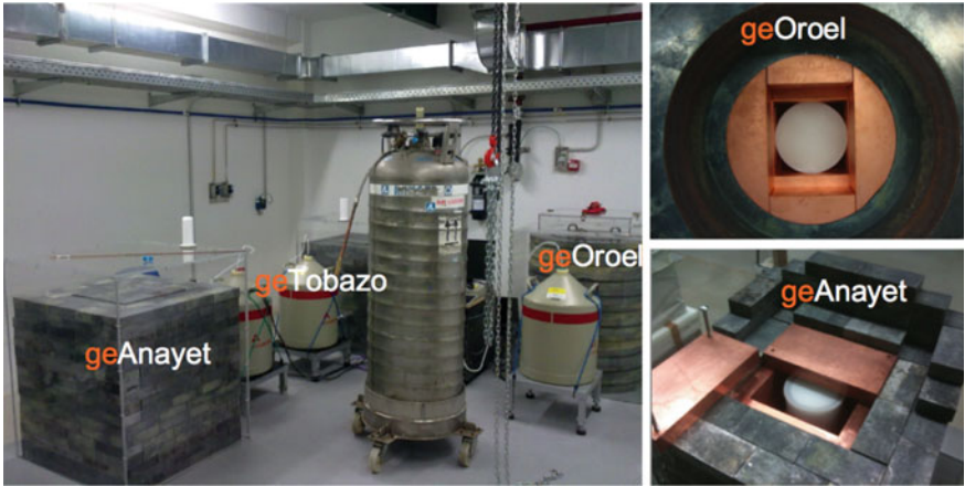
Fig. 5.32 Pictures of HPGe detectors in LSC (left) and of two of the HPGe detectors containing a marinelli in which the sample is kept during the measurement
