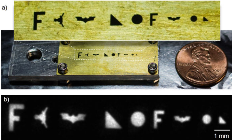
Fig. 8.22 (a) Photograph of the slide, for easy reference. (b) Composite image of the slide, again at 113 cm. Though the sizes are matched in this case, the magnification factor is 0.81
