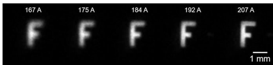
Fig. 8.20 Focusing sequence for the F-shaped aperture with the double peak correction field in place. Unlike in Fig. 8.11, we present the image right-side up. Image distance is 113 cm
