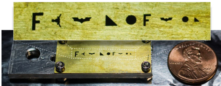
Fig. 7.15 Photograph of the slide used as an object for the focusing experiment. The atom beam passes through shaped apertures, just as in an optical transmission mask. The goal of the atom lens is to refocus the beam and reproduce the original shape. The letter F is an excellent object for early investigations, since it is asymmetric in two dimensions and has a simple, recognizable structure. For more advanced tests, shapes like the Texas Longhorn offer more detail and a broader range of size scales. The Batman logo, which is objectively cooler-looking than the version in Chapter 6, is included primarily to impress members of the opposite sex
