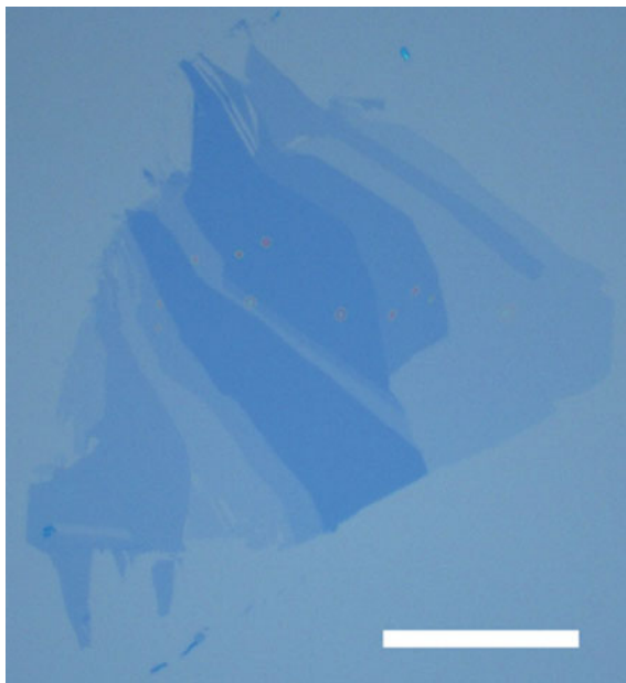
Fig. 3.7 Regions of mechanically exfoliated single-layer, bilayer and few-layer graphene. Also visible are bubbles characteristic of the mechanical exfoliation technique. Scale bar 100 \mu\text{m} . Picture and sample by Francisco J. Rodriguez, used in Chap. 5
