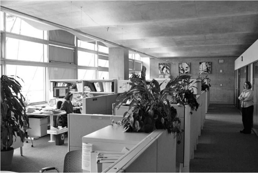
Figure 7.3 In the San Francisco Federal Building, north-facing windows permit work by daylight with only minimal use of electric lights (Morphosis, architect). Windows at top and bottom open to naturally ventilate the building. Credit: James S. Russell
