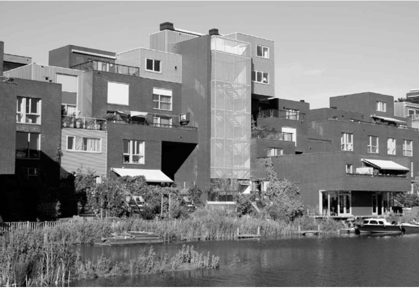
Figure 5.3 This new quarter in Amsterdam, called Ijberg, created a wildlife-rich water edge of vegetation, a model that can be used along streams to slow water flow and reduce flooding. Credit: James S. Russell
