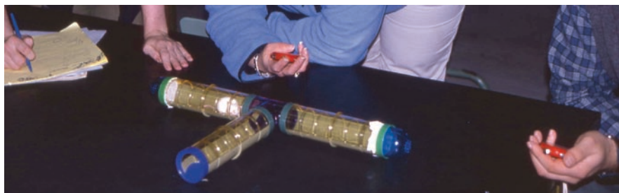
Two-way choice apparatus (T-maze) for testing mouse responses to odors of conspecifics
