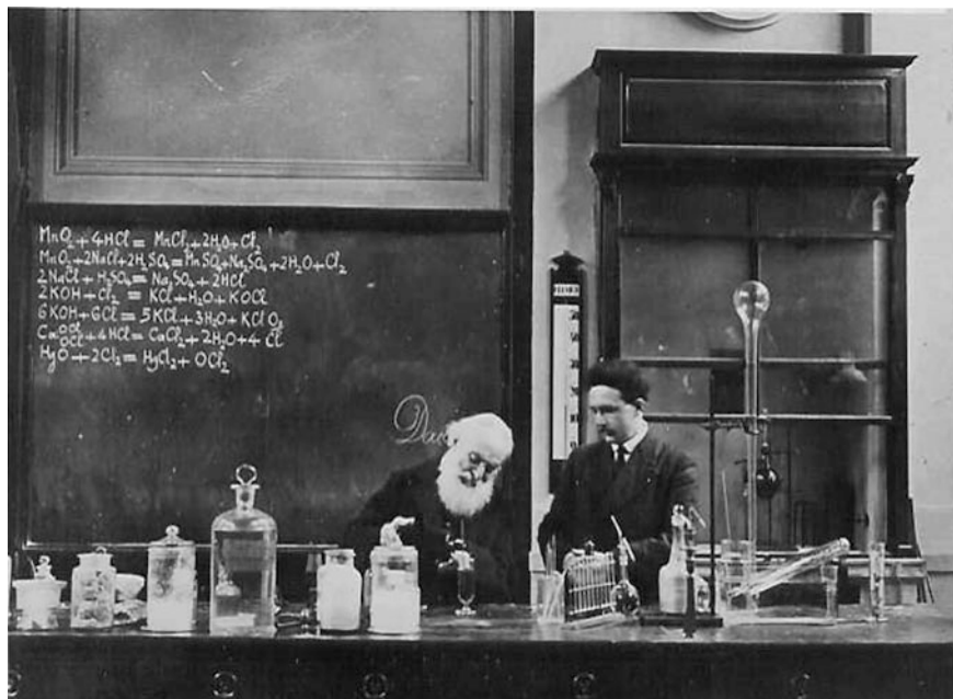
Fig. 4.3 Hugo Schiff ( left ) preparing a chlorine demonstration with his student, Guido Cusmano, ca. 1910–12. Note the fume hood on the right ; the preparation room is accessed by lifting the movable blackboard. Courtesy of Chemical Heritage, University of Florence
