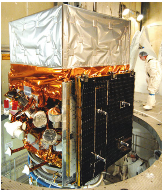
Fig. 2 The Fermi satellite during pre-launch testing [19]. The LAT instrument is visible on top of the spacecraft with the GBM detectors positioned at the lateral sides
