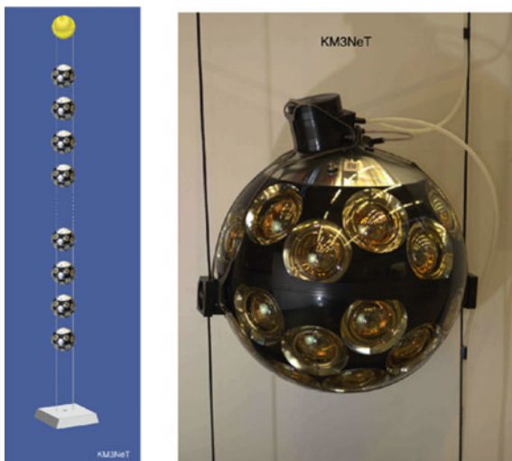
Fig. 44 A scheme of the detection string ( left ), the DOM held by two parallel ropes ( right ). Attached to the ropes is visible the vertical electro-optical cable, a pressure balanced, oil-filled, plastic tube that contains two copper wires for the power transmission (400 VDC) and 18 optical fibers for the data transmission
