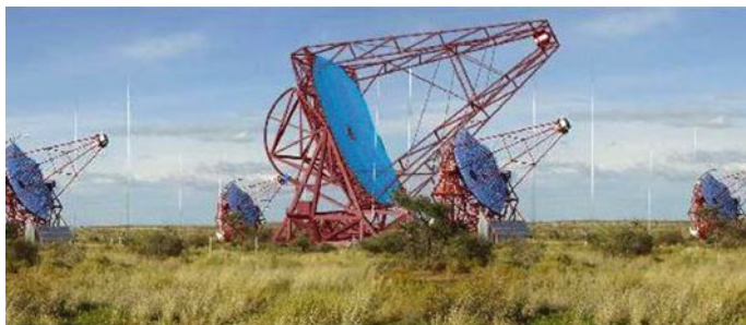
Fig. 3 The HESS system of four 13 m diameter Cherenkov telescopes. While this system has been operating in Namibia since 2003, the 28 m diameter telescope has been operating since 2012
