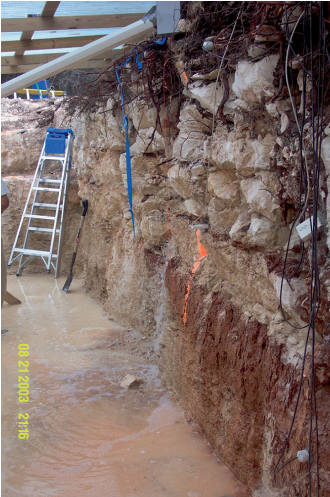
Figure 2 Photograph of a trench at the downslope end of an experimental hillslope receiving simulated rainfall. The trench is designed for capturing and measuring shallow subsurface flow as well as monitoring soil moisture at various depths
