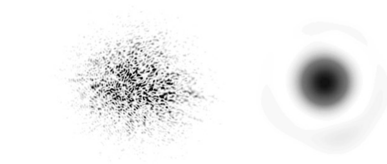
Fig. 4.10 Speckle images of a single point-like star in the visible ( on the left ) and in the mid infrared at 10\ \mu\text{m} ( on the right ) under identical atmospheric conditions on an 8-m telescope. In the 10\ \mu\text{m} image, parts of the first diffraction ring can be seen. The envelope of the speckle image has about the size of the seeing disk. A simulation for atmospheric turbulence was used to produce the images
