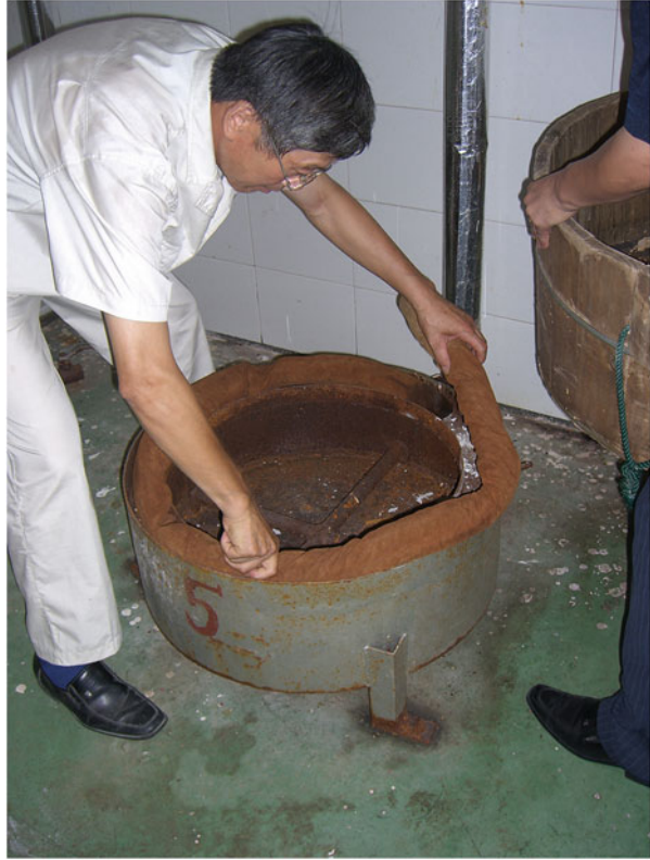
Fig. 4.2 Equipment for steaming sticky rice: vapour distribution
