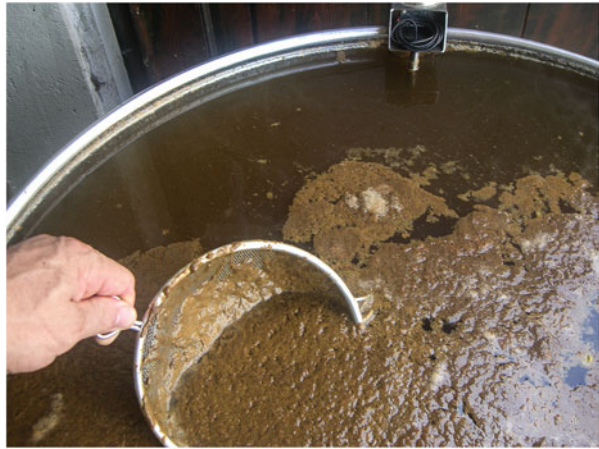
Fig. 4.5 Removal of fouling formed during the heating of grape must
