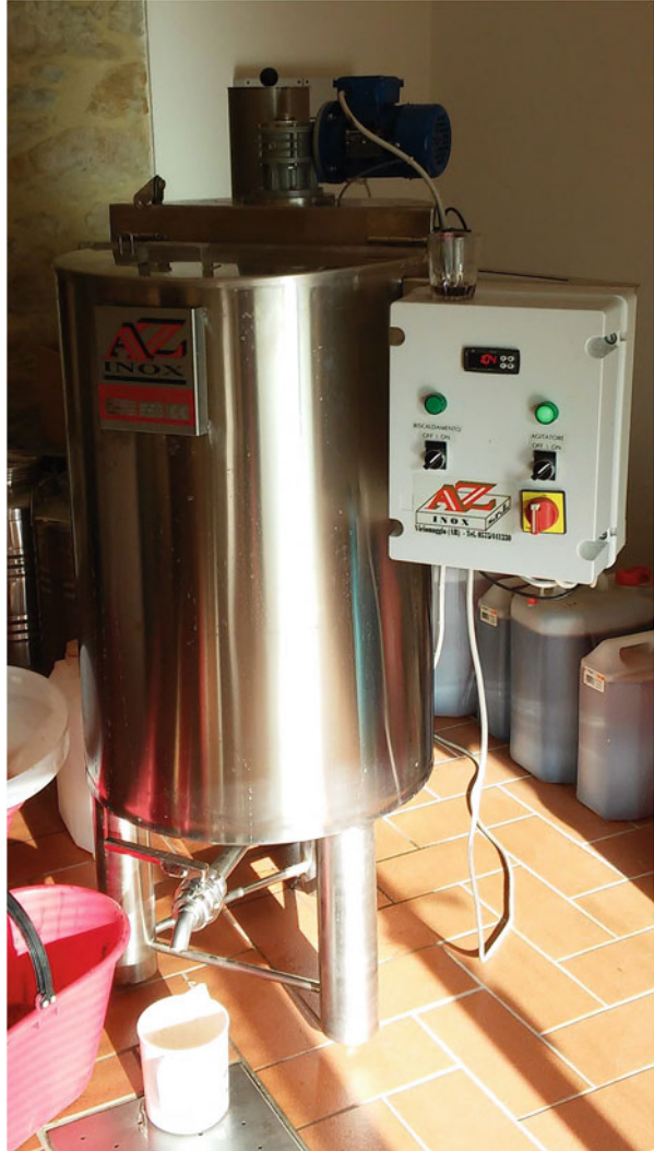
Fig. 4.3 A small pasteurisation device used for cooking grape must
