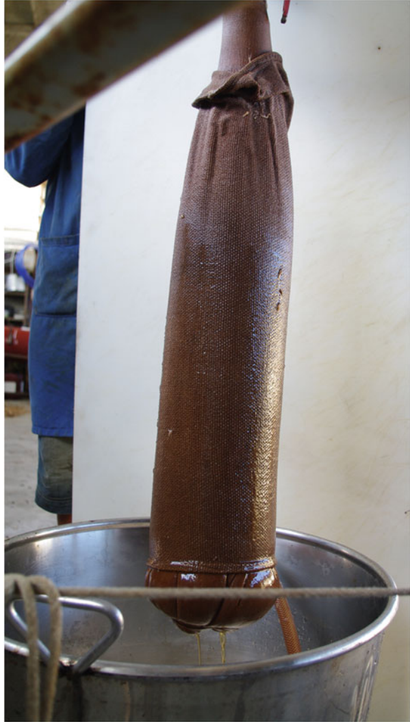
Fig. 5.5 Traditional filter cloth to remove lees after alcoholic fermentation
