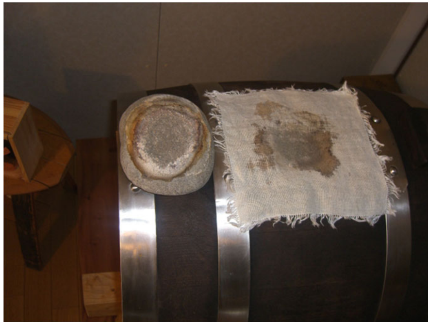
Fig. 4.7 Barrel with a river stone used to cover the bunghole. The granular sand released by the solubilisation of the river stone carbonate is evident on the cloth
