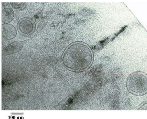
Fig. 7 Cryo-TEM picture of vesicles formed by a PMAA 49 - b -PDMAEMA 11 ampholytic copolymer in water at pH = 9 (Reprinted with permission from Ref. [134])
