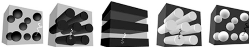
Fig. 15 The classical morphologies in block copolymer systems (With kind permission from Springer Science and Business Media [25])
