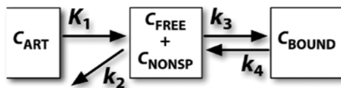
Fig. 3 Three basic PET kinetic models C_{\text{ART}} = concentration of nonmetabolized free tracer in arterial plasma
