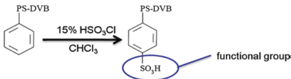
Fig. 6.10 Sulfonation reaction of polystyrene-divinylbenzene and sulfone groups characterized using FTIR-spectroscopy
