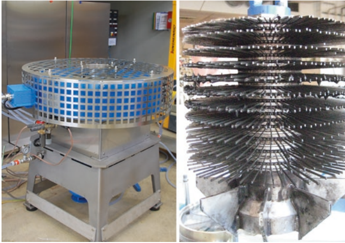
Fig. 8.3 The industrial-scale MEC ( left ) with the blue electromagnet installed around the machine; the machine is fed from the bottom and discharges at the top; a window is installed in the top to allow study of particle deposits; the wire matrix after cleaning ( right )
