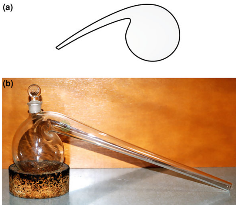
Fig. 6.7 Illustration of a basic early retort (a) and a photo of a modern glass retort (b)
