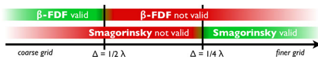
Fig. 2. Ranges of validity for the Smagorinsky model and for the \beta FDF model for a wave of wave-length \lambda according to [11]. There is no filter-size \Delta for which both models can be applied at the same time.
