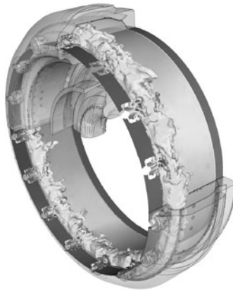
Fig. 3. Translucent part of the geometry along with pressure fluctuations on a cylinder containing all burners axis and a temperature isosurface representing the flame front, as obtained on the lighter grid.
