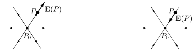
(a) charge Q_0 > 0 at the point P_0 (b) charge Q_0 < 0 at the point P_0
