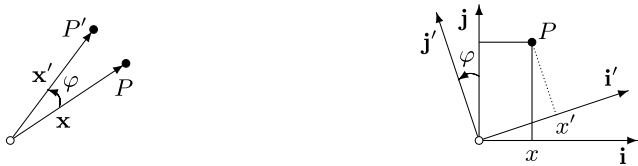
(a) active rotation of the point P (b) passive rotation of the point P
