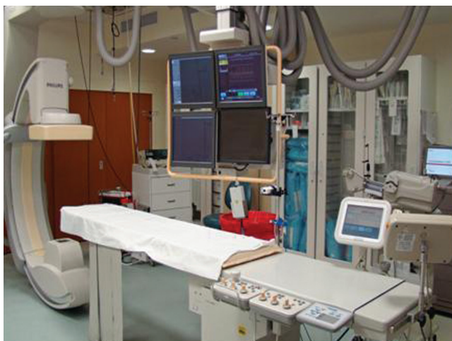
Figure 4.23 Cath lab with integrated intravenous ultrasound (IUVS) and fractional flow reserve (FFR) monitors.
