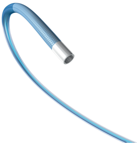
Figure 1.3 Illustration of a guiding catheter shows stiffer body; variable softer primary curve; wire braiding; atraumatic tip; large lumen (optional radio-opaque marker); lubricious coating. (Courtesy of Boston Scientific, Inc., Boston, MA.)
