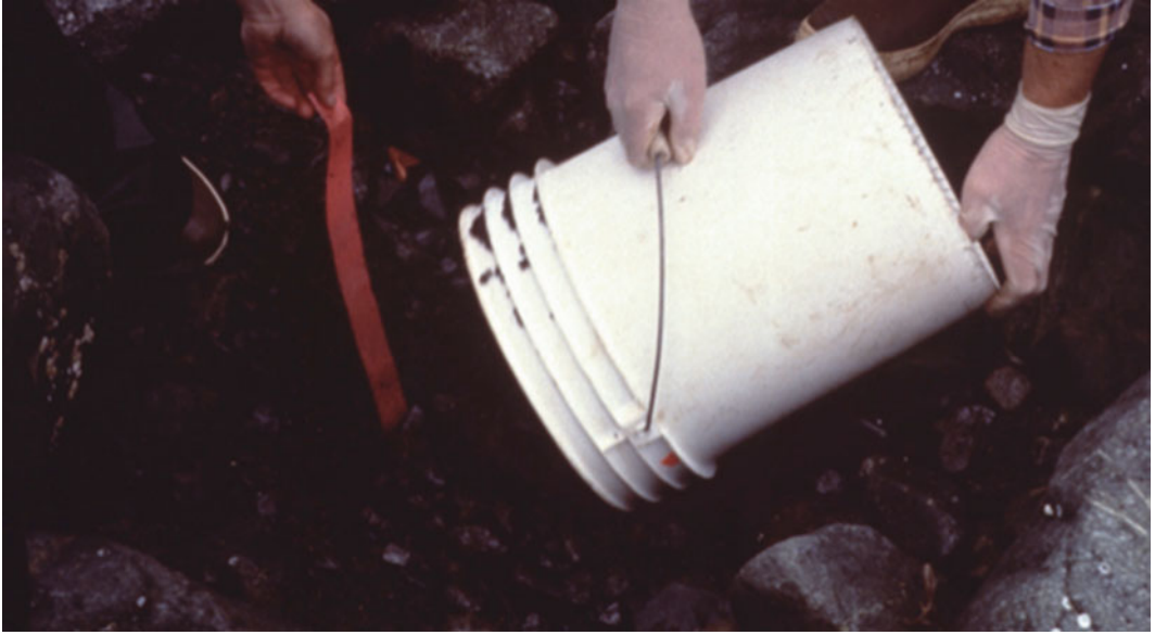
Fig. 5 Subsurface sampling – material removed to get to the appropriate depth was temporarily stored in a bucket to prevent contamination of surface areas to be sampled later and marked with surveyor's tape so that the area would not be resampled later
