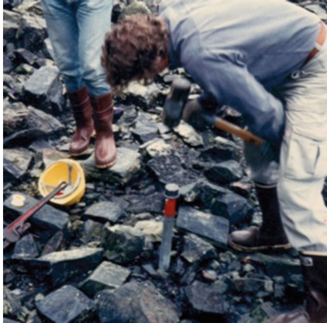
Fig. 3 Installing a sampling well on a shoreline in Prince William Sound. A slotted steel well is being driven into the sediment so that water flow within the shoreline material is only minimally affected. Note the use of safety glasses
