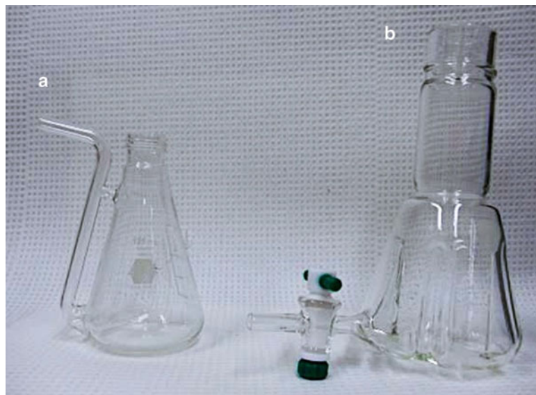
Fig. 1 “Swirling” flasks for USEPA dispersant testing. (a). The classic swirling flask (USEPA 2006) without baffles and with the drain tube extended to above the top of the flask. (b) The baffled flask of the recent USEPA proposal (USEPA 2015), with vertical baffles and a stopcock at the bottom. In use this flask sits level
