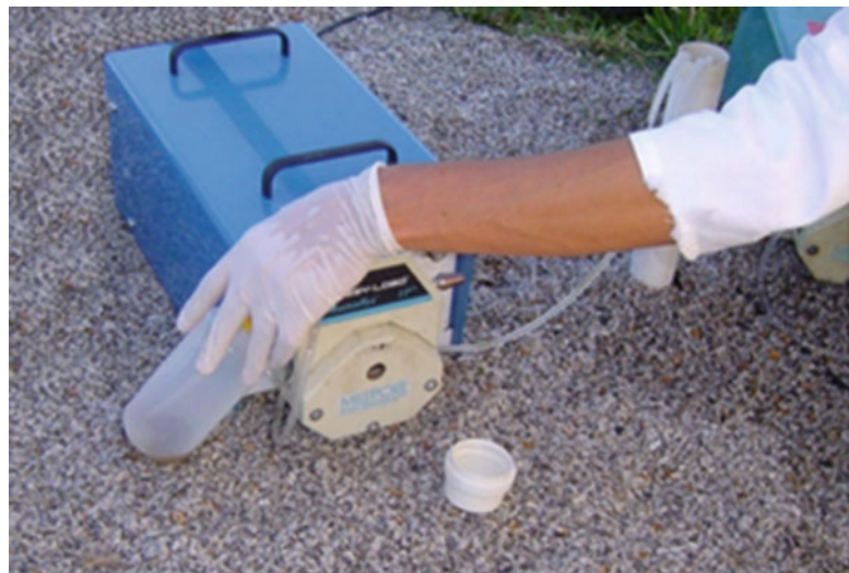
Fig. 7 Groundwater is sampled directly into HDPE flasks using a low-flow peristaltic pump and Masterflex Tygon tubing. Source: [61]
