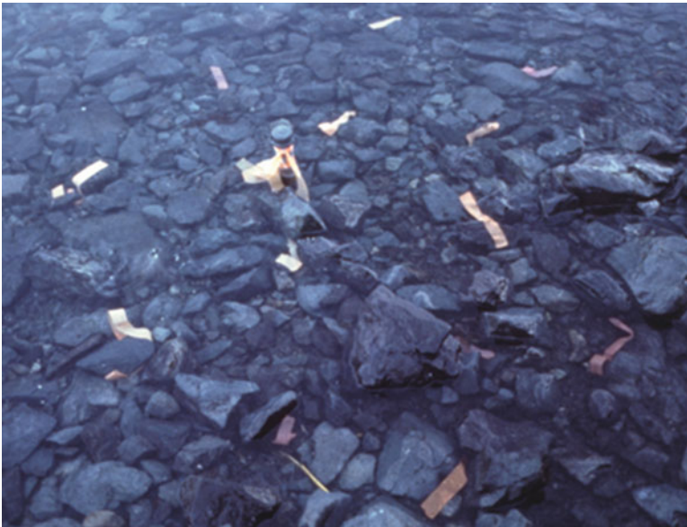
Fig. 6 Sampling area toward the end of the monitoring program. Samples had been collected around the sampling well and marked with surveyor's tape to prevent resampling
