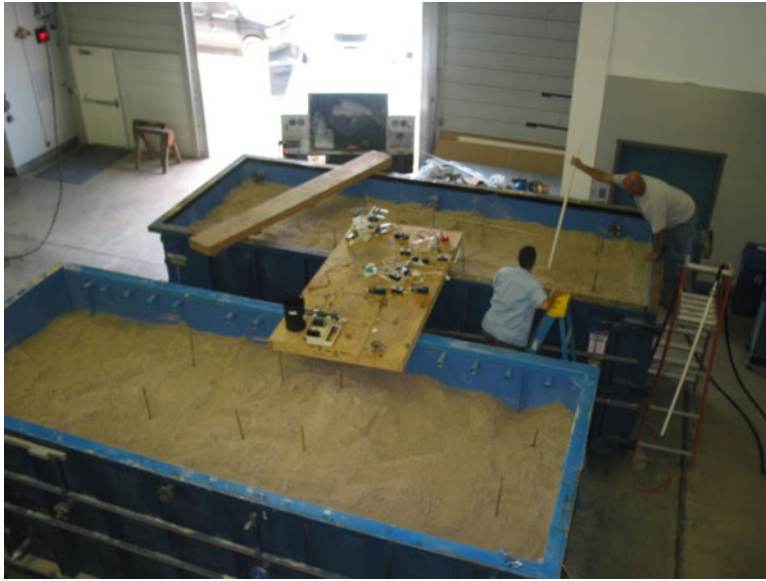
Fig. 3 Two metal tanks (5.5 m long \times 2.1 m wide \times 1.8 m high) filled with a non-contaminated sandy soil. Multiple internal sampling or injection points (0.6 and 1.3 cm ID, respectively) were installed using stainless steel tubing during tank packing. Source: [54]
