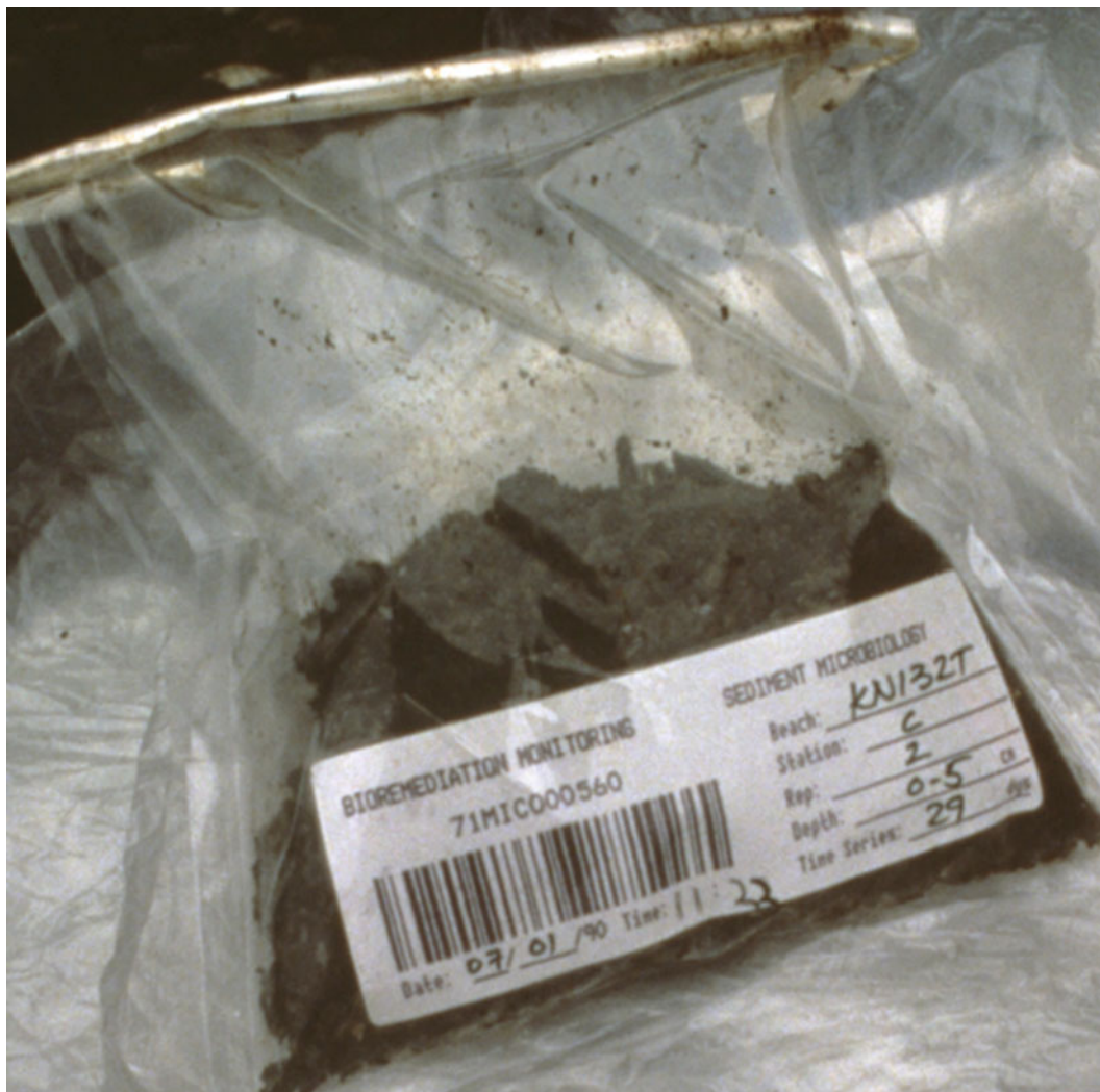
Fig. 7 A sediment sample for microbial analysis. A robust sample-labeling system was an important part of assuring that a reliable chain of custody was maintained
