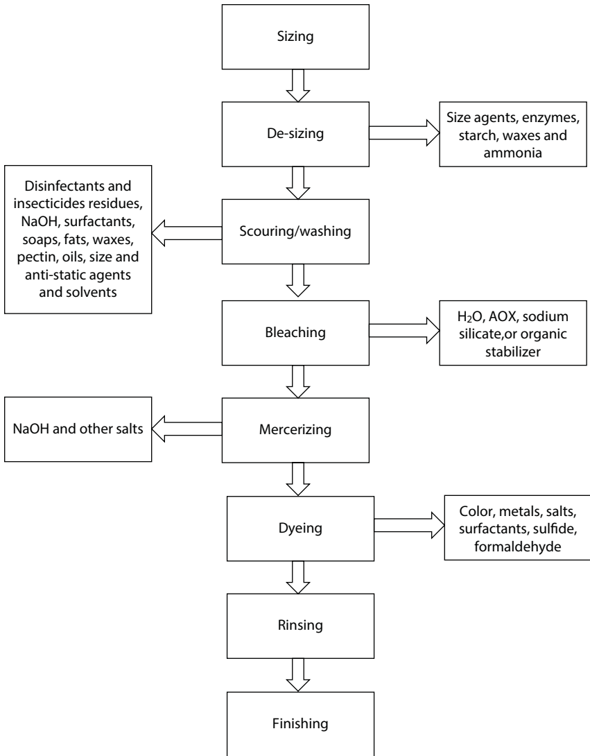
Figure 2.2 A description of the individual operations that are performed on cotton textile and the main pollutants that result from each operation.
