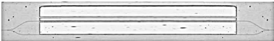
Fig. 9.16 Asymmetric Mach – Zehnder interferometer with the active region localized in both arms
