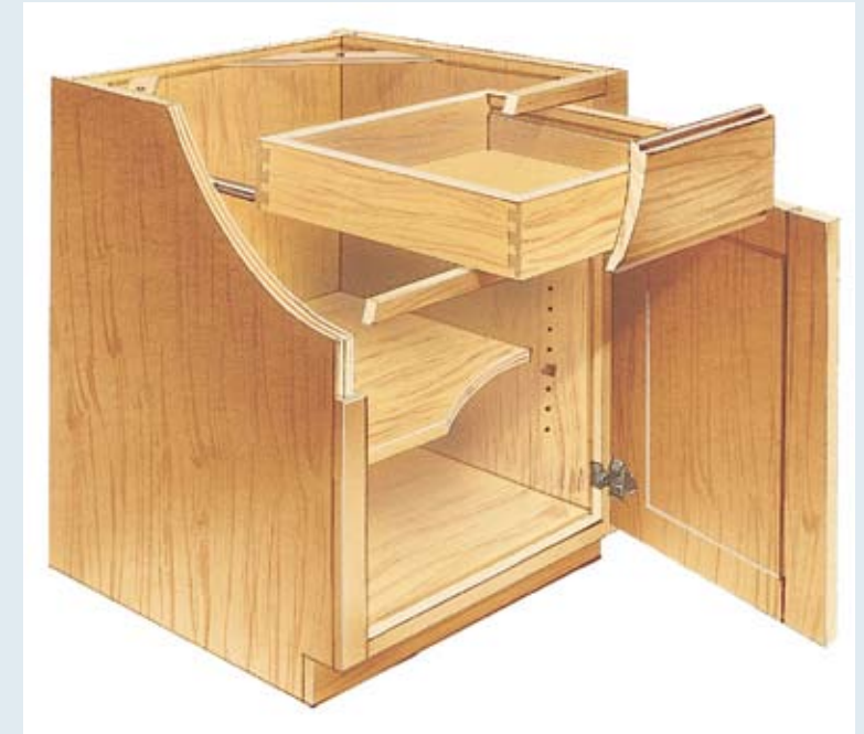
Face-frame cabinets have openings that are completely surrounded by face frames made of vertical stiles and horizontal rails. They give kitchens a traditional look.
