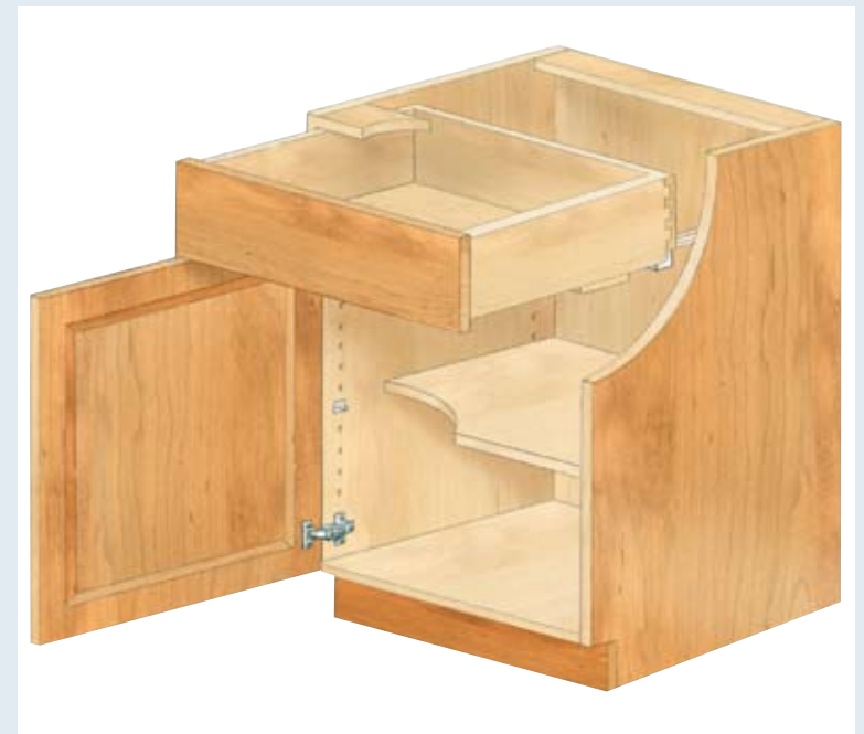
Frameless cabinets , sometimes called "European-style," are more contemporary. Because they have no face frames, frameless cabinets offer slightly more storage space than framed cabinets. The doors and drawers on frameless cabinets cover the entire unit.
