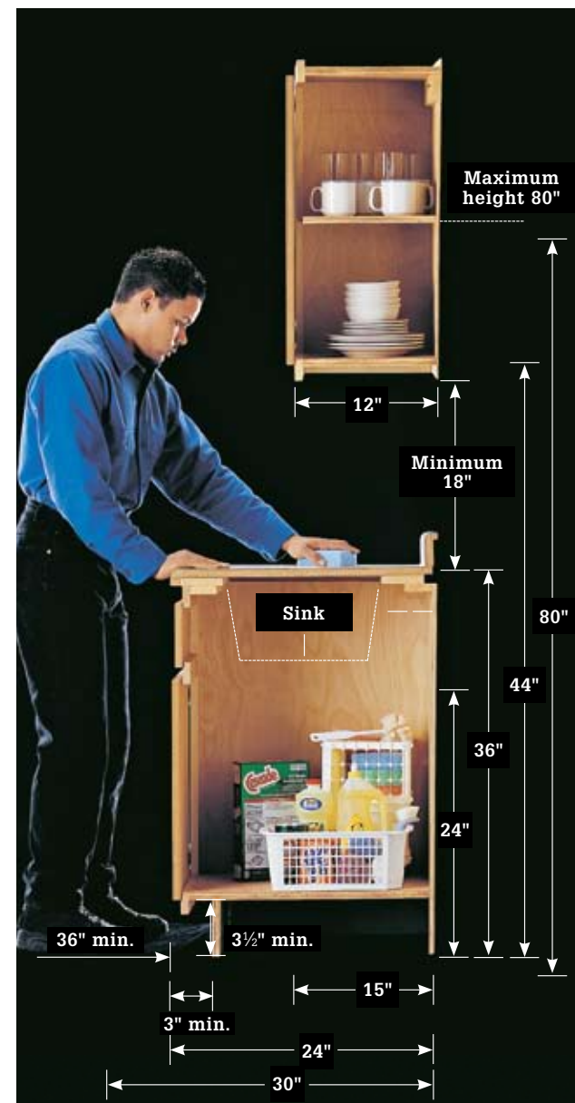
Dimensions and positions of cabinets follow accepted design standards, as shown here.
