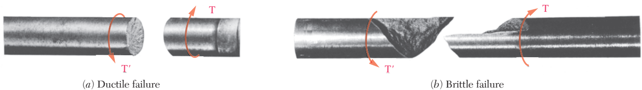
Photo 3.2 Shear failure of shaft subject to torque.
