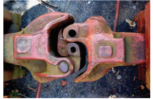
Photo 11.1 The railroad coupler is made of a ductile steel that has a large modulus of toughness.
