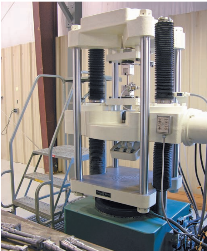
Photo 2.2 Universal test machine used to test tensile specimens.
