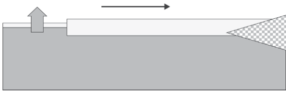
Fig. 3 One-dimensional thermal–mechanical lake ice model. Mechanics opens a lead, ridging takes place on the windward side, and new ice forms in the lead
