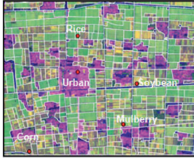
Fig. 3. A color composite of SPOT5 bands 4(SWIR), 1(green) and 2(red) with the digitized agricultural field boundaries overlaid
