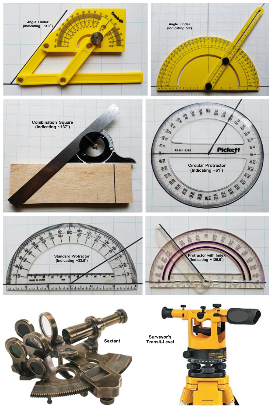
Fig. 10.11 Various types of flexible angle measurement devices
