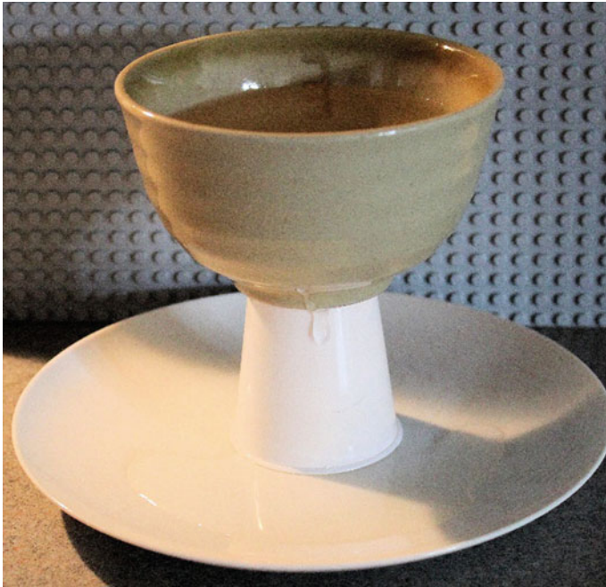
Fig. 8.2 Model of outflow water clock 0.99 mm hole in basin allows water to drip out at controlled rate Markings in basin indicate water level at 3 minute intervals
