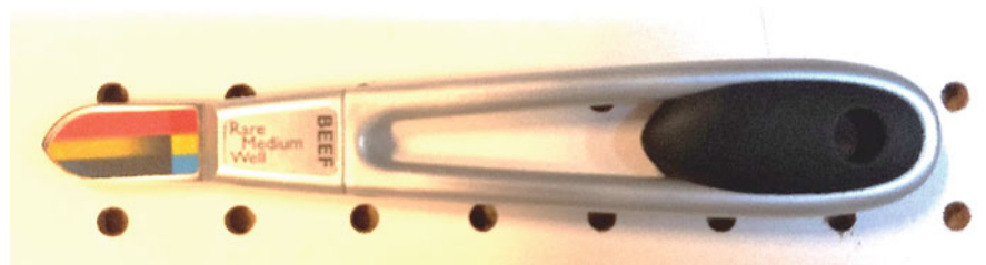
Fig. 9.11 Color-changing meat thermometer. When inserted into meat, color change on blade at left indicates the temperature and “doneness” of the meat. Reading shown is medium-well
