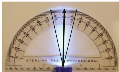
Fig. 13.6 Graphical concept for apex angle of a narrow-beam light source
