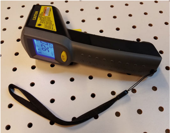
Fig. 9.8 An inexpensive spot infrared thermometer with laser aim
