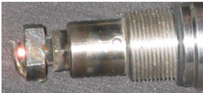
Fig. 18.4 Optical igniter with optical discharge
