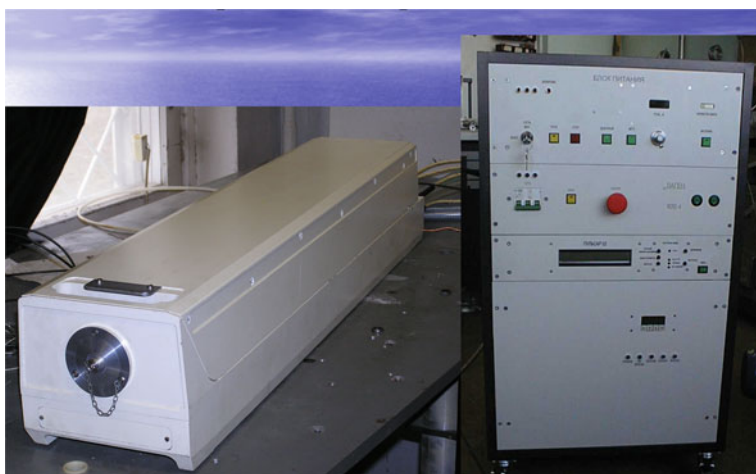
Fig. 18.2 Laser head and power supply
