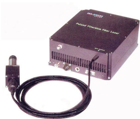
Fig. 18.3 Laser head YPL1/ 100/20
