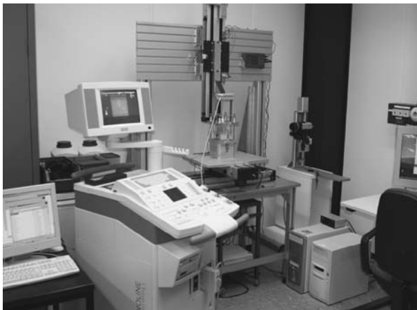
Fig. 6.11 The experimental setup to measure and reconstruct the shear modulus of phantom materials using ultrasound elastography
