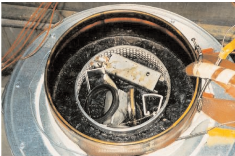
FIGURE 3.3 Macro-encapsulation is used to stabilize heterogenous waste or large objects for disposal. Typically, grout or a polymer is poured over the waste so that it is encased physically. There are few data on the long-term durability of macroencapsulated wastes. Source: DOE Richland Operations Office.
