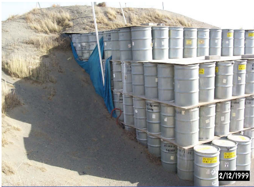
FIGURE 2.2 Since 1970, DOE has required that sites store TRU waste so that it can be retrieved easily. TRU wastes at Hanford, which is in a very dry region, are stored in earthen mounds. Source: DOE Richland Operations Office.
