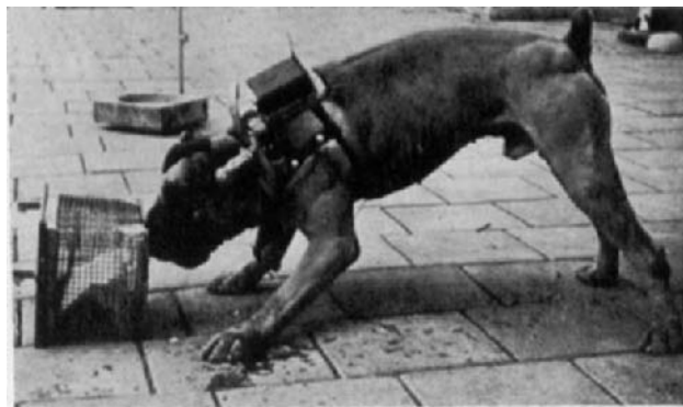
Fig. 1. The dog (German boxer) carries the 8 channel telemetering apparatus on his back. He is sniffing and biting at a meshwire container in which fish is placed. During this time the activities of 8 brain areas are recorded.
