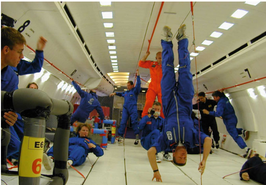
Fig. 16 During a parabolic flight on board the Airbus A300 ZERO-G during an ESA campaign, several experimental racks are visible to the left and the back while the author floats freely “upside down”. There is no “up” and “down” in weightlessness. (Photo: ESA)
