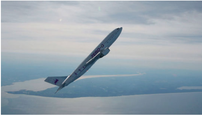
Fig. 17 The Airbus A310 ZERO-G during the pull-up. (Photo: Novespace—Eric Magnan/Airborne Films)
