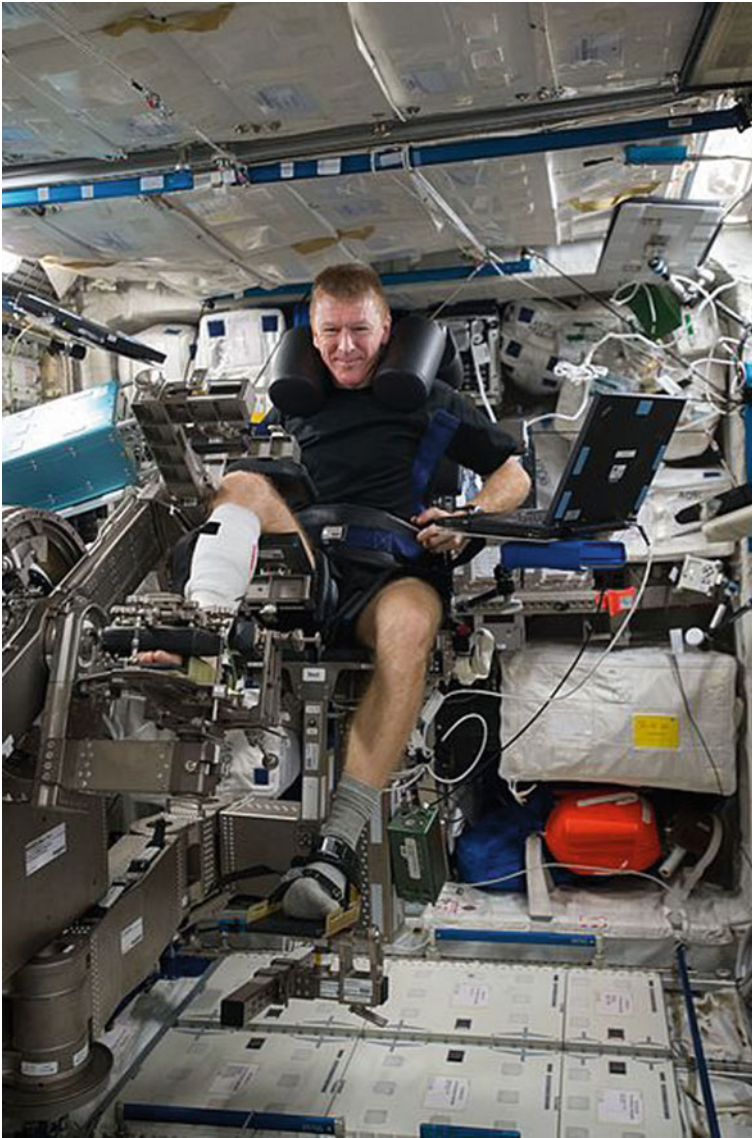
Fig. 38 British ESA astronaut Tim Peake operates the Muscle Atrophy Research and Exercise System (MARES) equipment inside the Columbus module. MARES is an ESA facility used for research on musculoskeletal, biomechanical, and neuromuscular human physiology to better understand the effects of microgravity on the muscular system (Photo: NASA/ESA)
