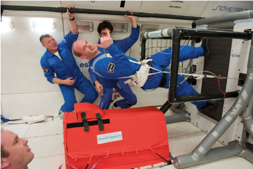
Fig. 39 ESA astronaut Alexander Gerst tests a running treadmill during parabolic flights on Airbus A300 under supervision of the author. Note the vertical position of the running surface. The entire treadmill setup was installed vertically due to the large vertical dimension of the treadmill and its subsystems, impeding its installation in a horizontal configuration. The subject ran toward the cabin ceiling in 0 g (there is no up or down in 0 g ...). He is lying on an elevated mat (in red) during the high g pull-up and pull-out phases (Photo: ESA)
