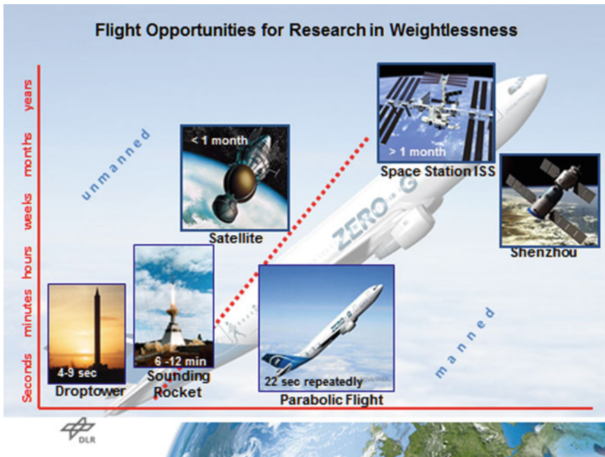
Fig. 26 Reduced gravity platforms accessible to microgravity researchers. (Credit: DLR)
