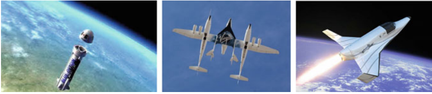
Fig. 19 Three suborbital facilities in development: (left) the New Shepard capsule with a reusable rocket (Credit: Blue Origin); (middle) the WhiteKnightTwo airplane carrying the SpaceShipTwo spaceplane (Photo: Virgin Galactic); (right) the Lynx spaceplane (Credit: XCOR)
