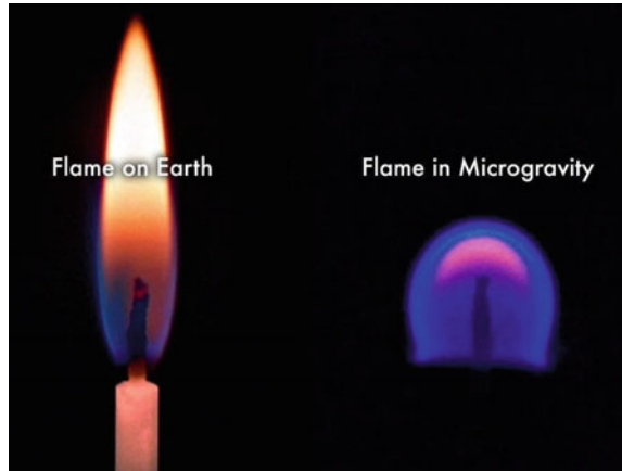
Fig. 29 Flames on ground in 1 g (left) and in microgravity in near 0 g (right). Notice the near-hemispherical shape of the flame in microgravity with the reddish-purple part on top due to some convection caused by small perturbations in the microgravity environment. (Photo: NASA)
