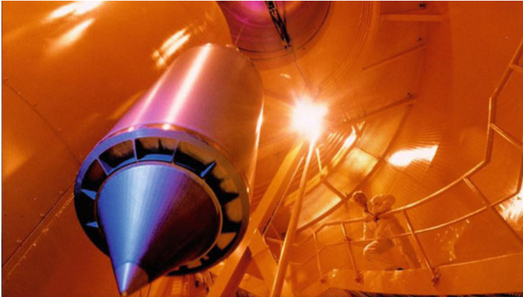
Fig. 14 The experimental capsule of 81 cm diameter and 1.85 m high, lifted to the ZARM tower top. The capsule aerodynamic profile and the fall in vacuum of 10^{-5} bar allow to minimize to the extreme the atmospheric friction. The decelerating container of 8 m high, filled with polystyrene balls, is seen to the left. (Photo: ZARM)
