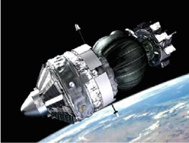
Fig. 23 On a low Earth orbit at approximately 300 km altitude and 62.8° inclination for 12 days in September 2007, the Foton M3 capsule carried a 400 kg European experiment payload with experiments in fluid physics, biology, crystal growth, radiation exposure and exobiology. (Credit: ESA)
