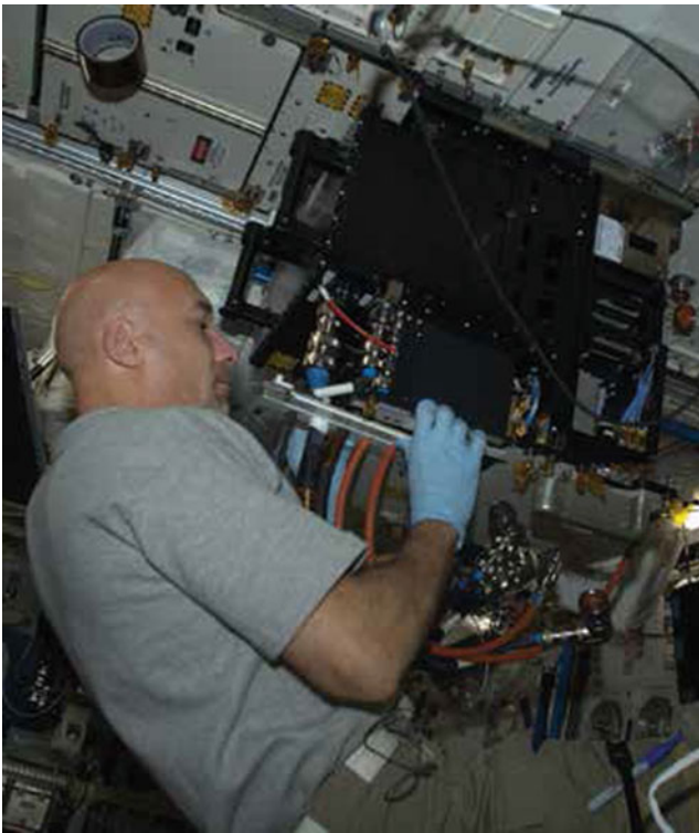
Fig. 22 ESA astronaut Luca Parmitano installing the FASES experiment in the Fluid Science Laboratory in the European Columbus Laboratory on the ISS in June 2013. (Photo: ESA)
