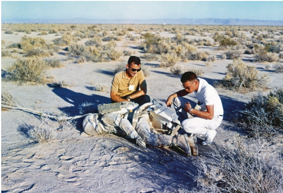
Young examines a manikin dressed in a pressure suit following a 1963 parachute ejection test. (Courtesy Ed Hengeveld)
