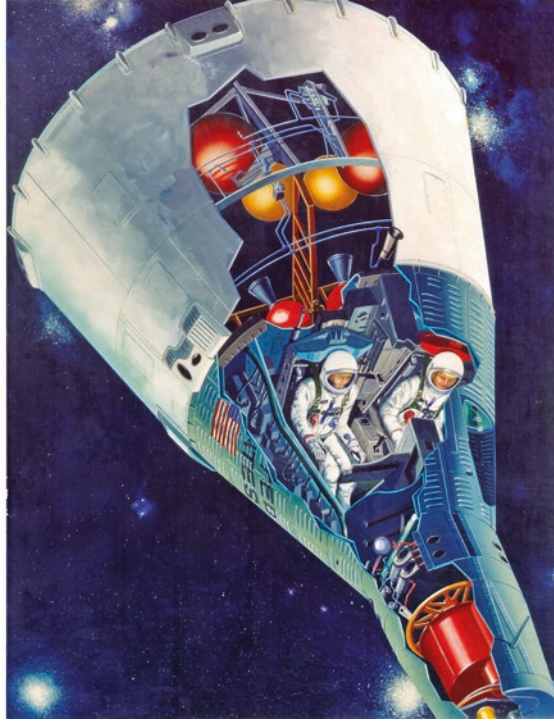
Gemini cutaway revealing the Rendezvous and Recovery section at the front, small end of the spacecraft, the two-astronaut crew compartment, the Retrograde section and the Adapter Module at the rear.
