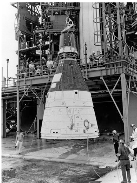
[Left] March 5, 1964: The Gemini 1 spacecraft is carefully hoisted off the ground at the base of Pad 19 at Cape Kennedy for mating to its Titan II launch vehicle. [Right] Gemini 1 in the White Room Pad 19. In the background receiving early first-hand experience of Gemini launch pad procedures are (from left) astronaut Elliott See, engineer Guenter Wendt the McDonnell Aircraft Corporation pad leader, with astronaut Neil Armstrong far right. Nine months later, Armstrong and See would serve as the backup crew to Gordon Cooper and Pete Conrad for Gemini 5. (Images courtesy Ed Hengeveld)
