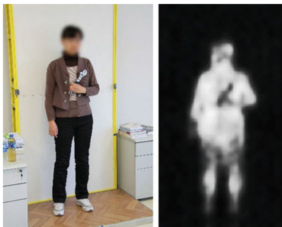
Fig. 25 Detection test of hidden objects under human clothing (the target is a mental wrench, left one is optical picture while right one is millimeter-wave picture)
