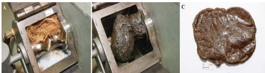
Figure 6.3 Processing of composites in the mixer thermokinetics (A and B) and composites of PP reinforced with coconut fibers (C).
