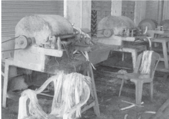
Figure 11.3 Decorticating machine used for mechanical fiber extraction. (From A. V. R. Prasad, K. M. Rao, G. Ragavirasulu, Indian Journal of Fibre and Textile Research , 2009 [30]. With permission from Indian Journal of Fibre and Textile Research ).
