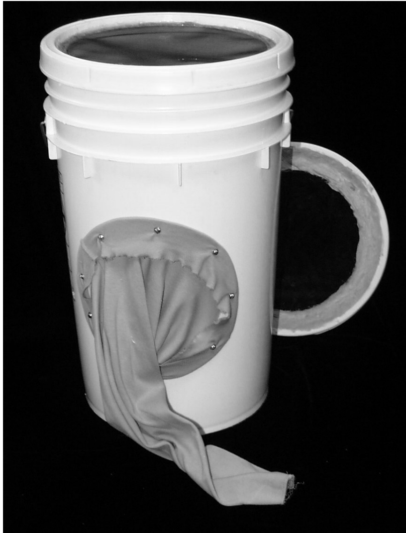
Figure 45. Bucket cage with screen top (optional clear pane top shown in background) and sleeve access.
