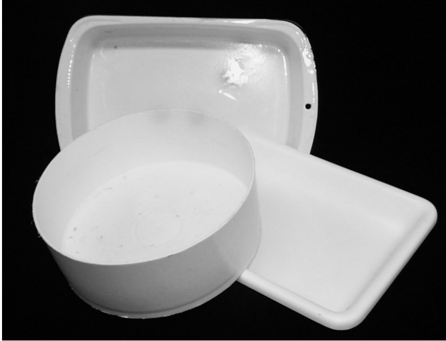
Figure 8. Several types of white pans, tray at front left was made from the bottom of a bucket.
