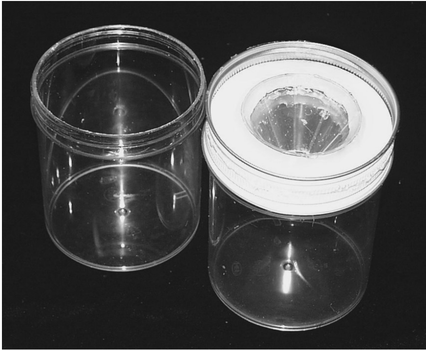
Figure 70. An emergence trap constructed from two jars, the jar on the left fits on top of the other jar when in use.
