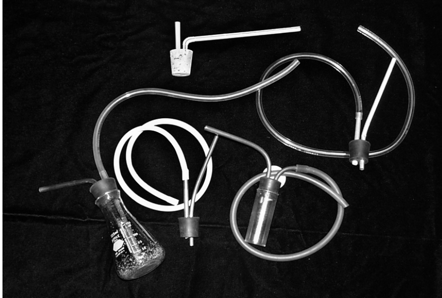
Figure 2. Aspirators fitted with collecting receptacles.
