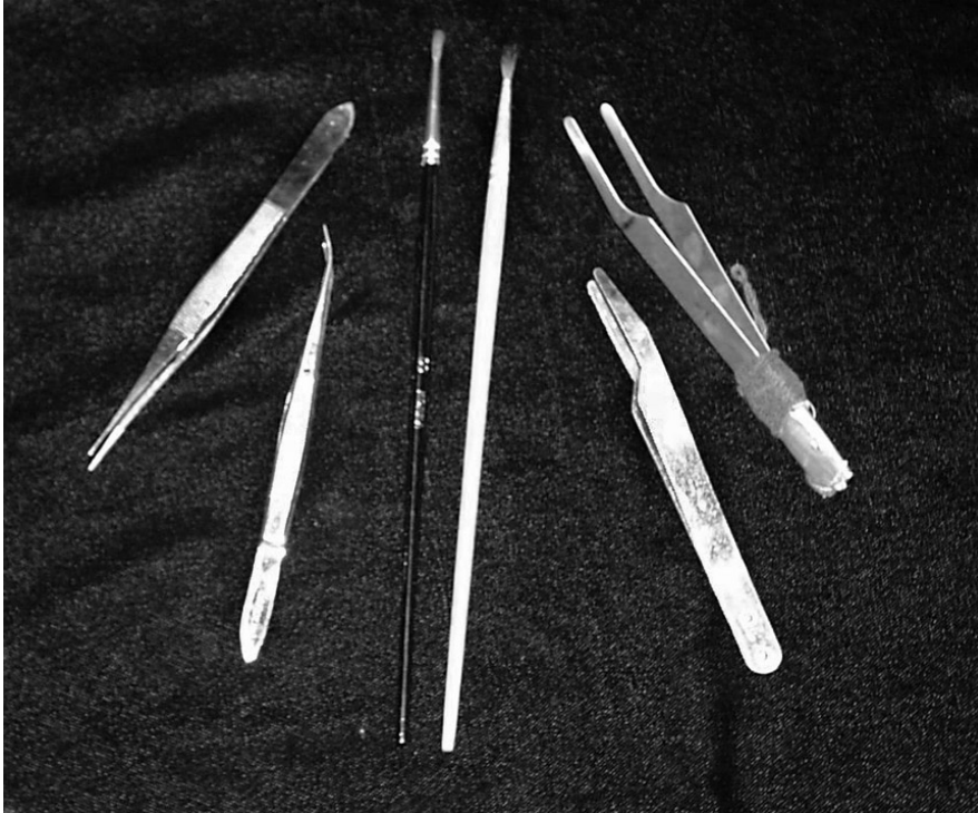
Figure 65. "Tools of the trade" (from left) forceps, fine point paint brushes and "soft touch" forceps.
