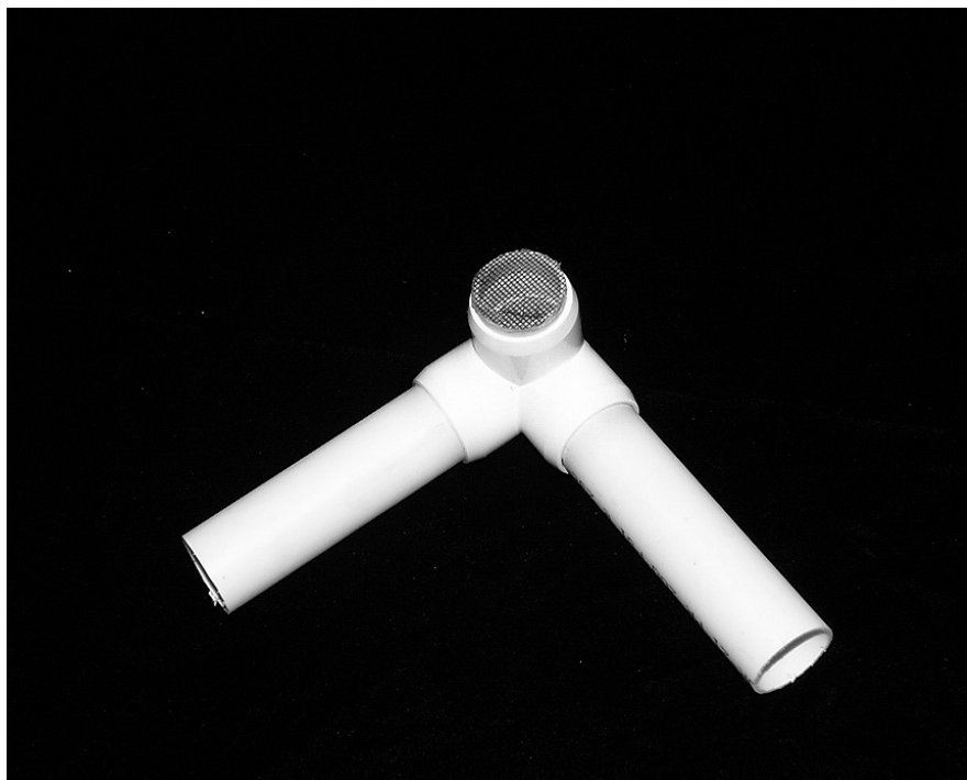
Figure 68. A device for holding large insects while marking, a vacuum is applied to one end of the device holding the insect in place on the screened area (upper center).
