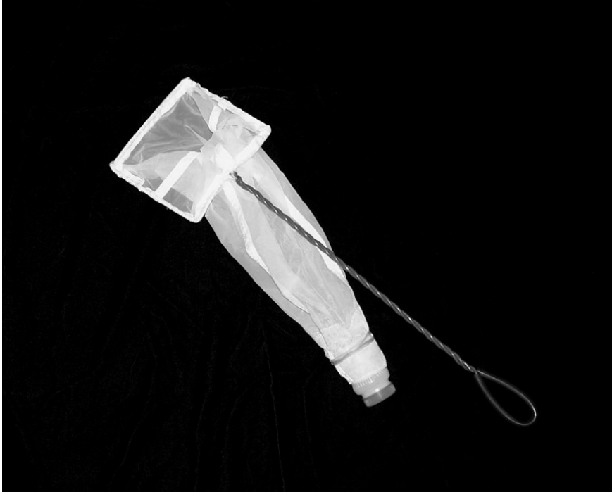
Figure 13. A plankton net constructed from an aquarium net.
