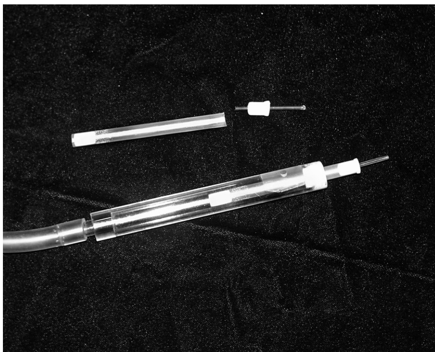
Figure 3. Micro-aspirator for collecting tiny organisms.
