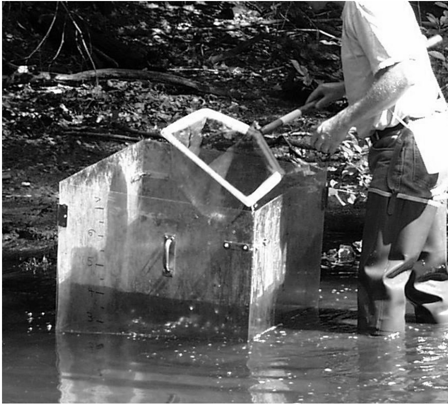
Figure 19. An aquatic sampling frame being used in a pond.
