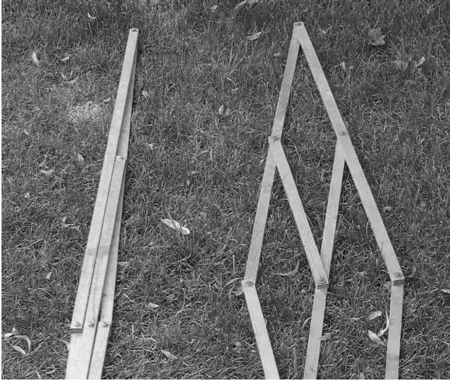
Figure 18. Detail of sampling frame construction illustrating accordion folding action.
