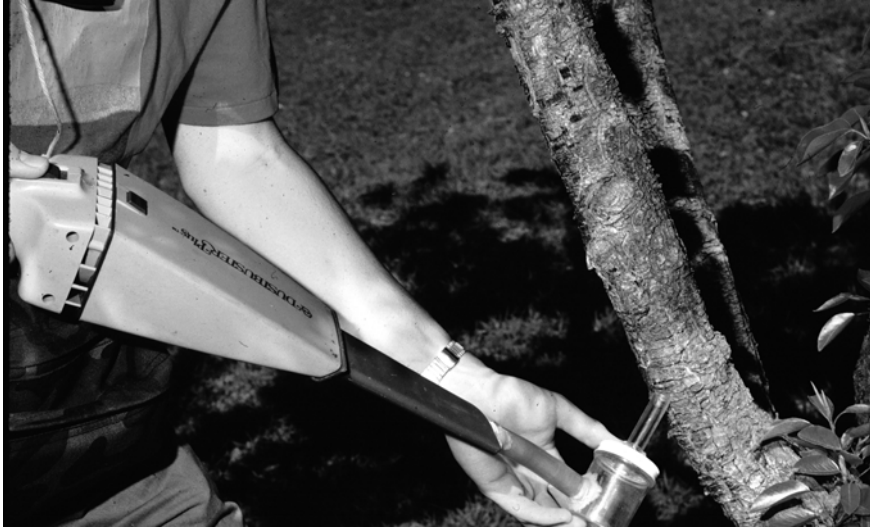
Figure 6. Vacuum collector being used to collect ants from a tree trunk.
