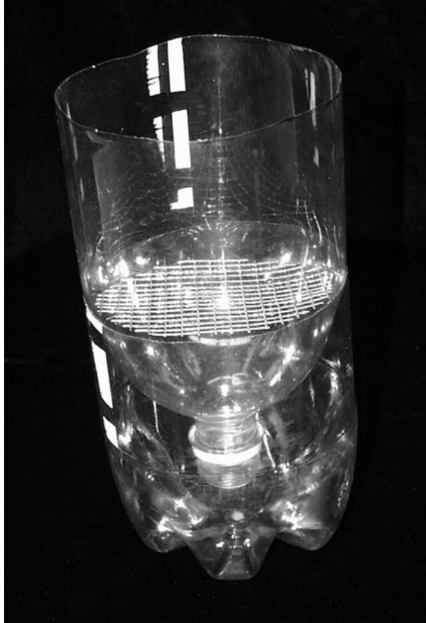
Figure 38. A Bursese funnel made from a soda bottle. Alcohol should be placed in the base to kill insects that fall from the sample.
