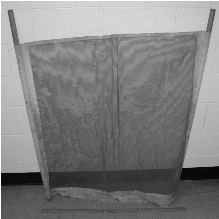
Figure 20. A standard kick net, the ruler at the bottom is one meter long.
