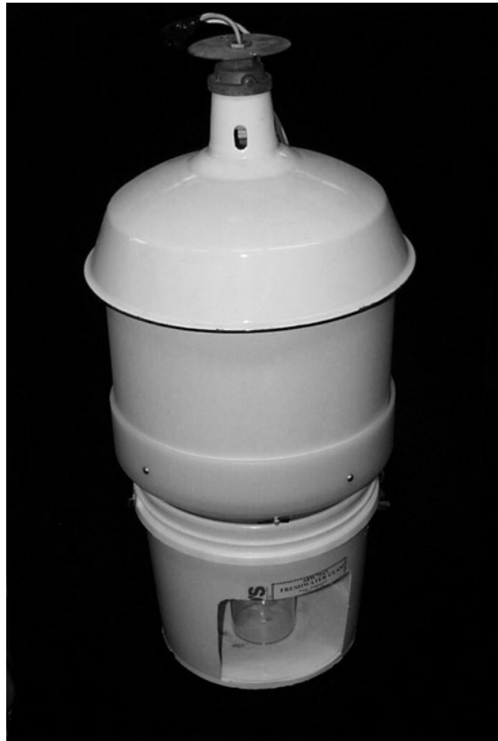
Figure 40. A large Burslese funnel made from a plastic bucket, aluminum flashing and an old light fixture.
