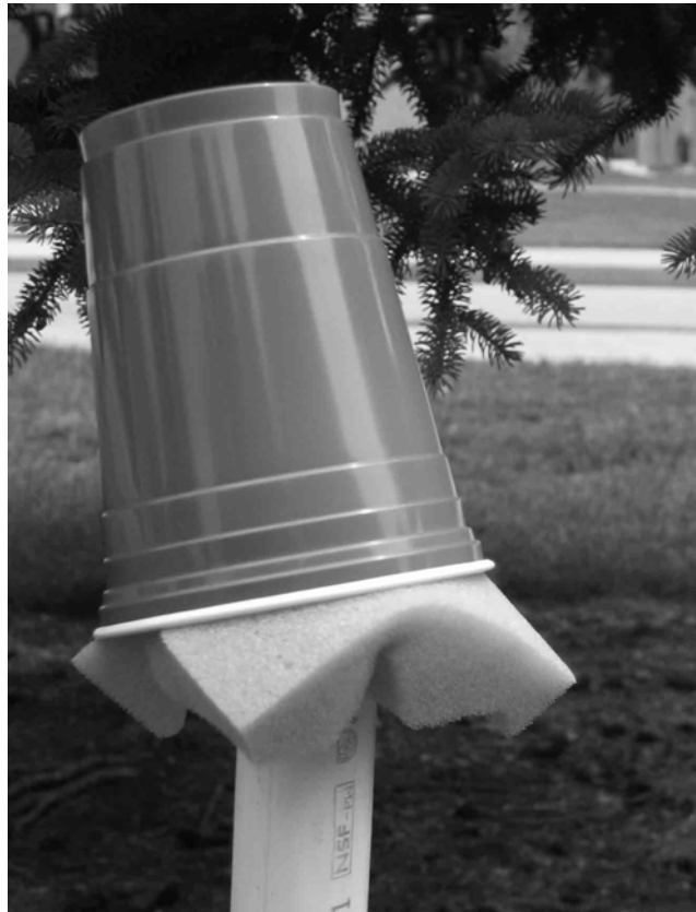
Figure 34. A sticky trap made from a plastic cup. Foam rubber holds the cup in place on a stake made from PVC pipe.
