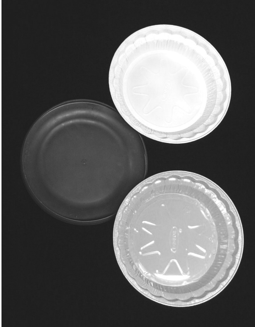
Figure 23. Pan traps made from painted pie tins (upper and lower right) and a flying disc (left).
