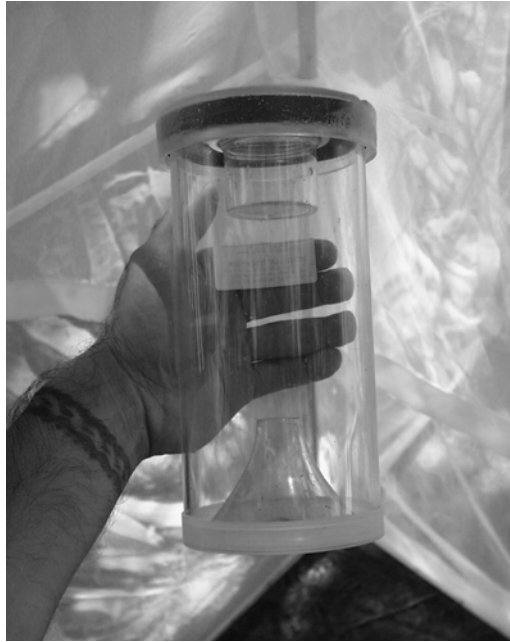
Figure 27. Collection chamber of a Malaise trap, note the inverted funnel in the lower portion intended to trap insects in the chamber.
