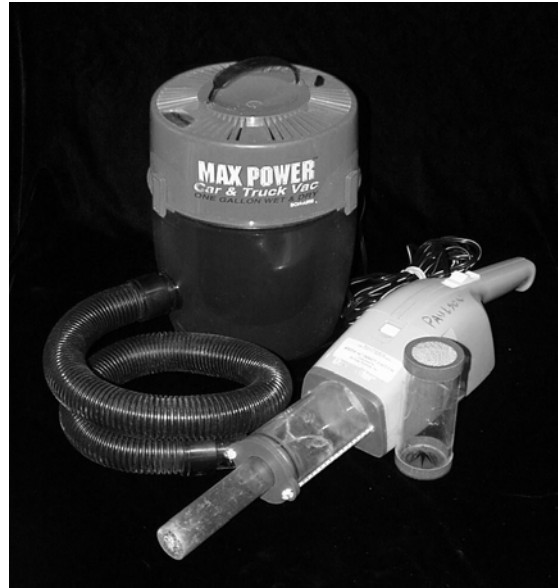
Figure 7. Canister style vacuum collector (left) and commercially available dustbuster style vacuum collector (right)
