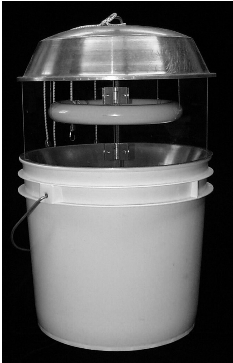
Figure 30. Light trap with bucket collection chamber.
