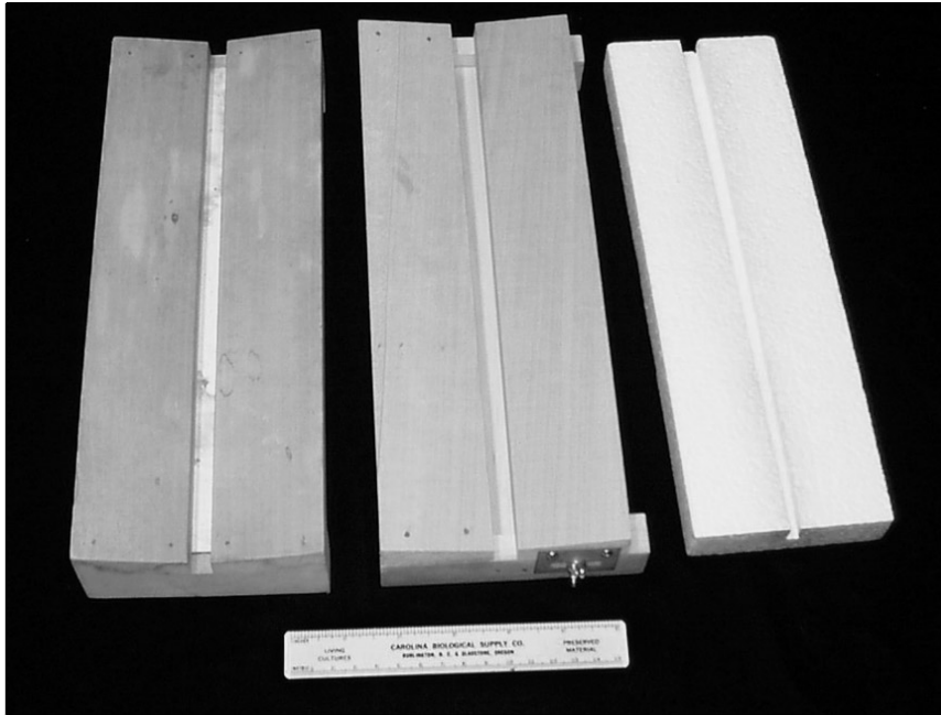
Figure 59. Spreading boards (left to right) homemade wooden, adjustable wooden made from commercially available kit, and commercially available Styrofoam board.
