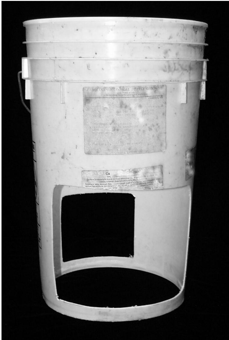
Figure 10. Surber-type sampler constructed from a plastic bucket, note that the net was left out of the photograph for clarity.
