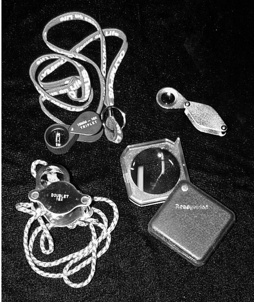
Figure 64. Types of magnifiers (clockwise from lower right); single plastic lens, doublet magnifier, 10X triplet magnifier and 15X triplet magnifier.
