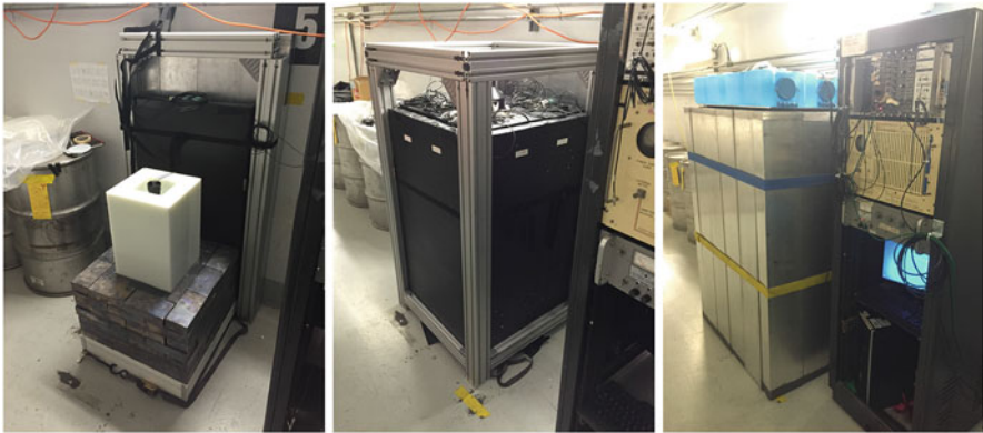
Fig. 5.2 Pictures of the \text{CE}\nu\text{NS} search detector deployment in June 2015 at the SNS. The leftmost picture highlights the innermost layers of HDPE used to reduce the background originating from NIN production in the surrounding lead (Chap. 4). The middle picture shows the setup once the aluminum frame was assembled. The right picture shows the full installation, including the NIM rack. Images courtesy of Juan Collar
