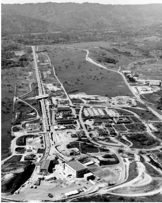
Fig. 6.2 Aerial photo of the Stanford Linear Accelerator (SLAC) around 1968. On the left is the approximately 3 km long linear beamline used to accelerate the electrons. The buildings for the particle detectors are in the foreground at the bottom left Source: U.S. Department of Energy
